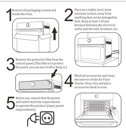
Upon first use, it is necessary to run the oven for 18 minutes at the highest temperature (230  $^{\circ}$ C) in order to sterilize and remove any manufacturing odor. The Air fryer Toaster Oven may emit an odor or smoke due to the heater's protective film.
