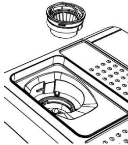
2. Rotate the internal grinding wheel counterclockwise out.
